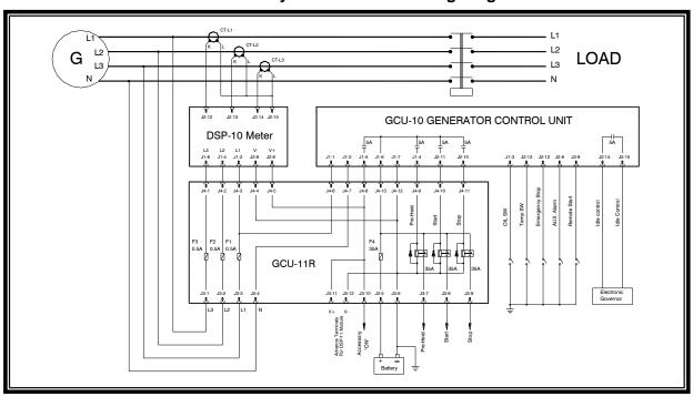
**Single Phase System Standard Wiring Diagram**
